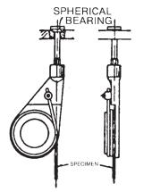
FIG. 5 Snubbing Device for Testing Wire
