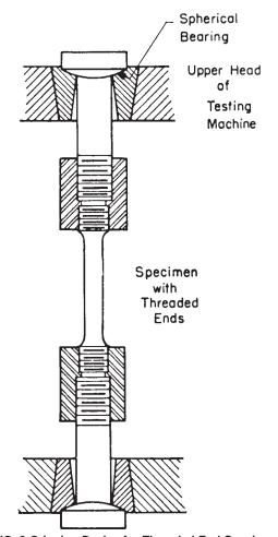
FIG. 2 Gripping Device for Threaded-End Specimens
