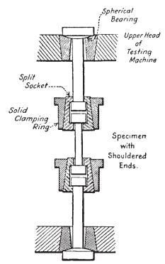
FIG. 3 Gripping Device for Shouldered-End Specimens
