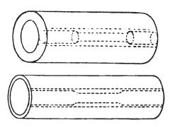
Note 1—The edges of the specimen shall be cut parallel to each other. FIG. 12 Location from Which Longitudinal Tension Test Specimens Are to Be Cut from Large-Diameter Tube
